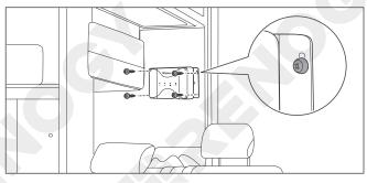
Place the battery charger against a flat surface and secure it with included screws.
