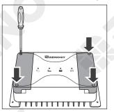
4. Remove the four screws on the protective cover and remove the cover with a phillips screwdriver.
