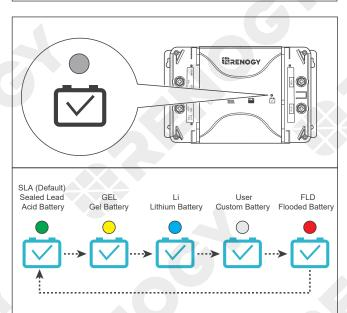
2. The Battery Type Indicator flashes different colors to represent different types of battery.
