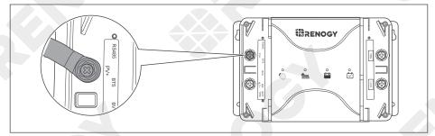
Connect the positive terminal of the solar panel to the Positive Solar Terminal (PV+) of the battery charger.
