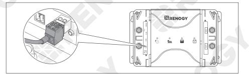
Insert the terminal block of the IGN Signal Wire to the Ignition Signal (IGN), and the bare wire terminal to the ignition of the vehicle.
