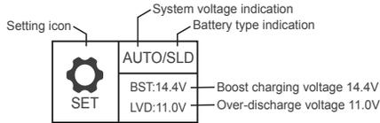
To enter the following settings, in the parameters setting screen press the Right arrow button.
