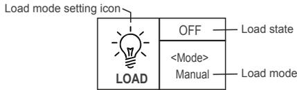
1. If the characters displayed on top of "<Mode>" are "ON", it indicates that the load is switched on
