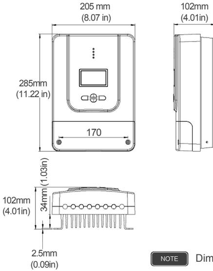
**NOTE** Dimensions in millimeters (mm)
