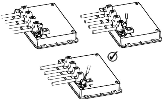
4. Insert the battery voltage sensor terminal block in the Batt Remote port. This is polarity sensitive. (Optional, requires a separate purchase).
