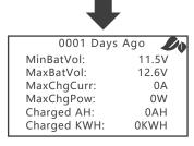
MinBatVol: Batteries lowest voltage for current day MaxBatVol: Batteries highest voltage for current day MaxChgCurr: Maximum charging current (Amps) for current day
