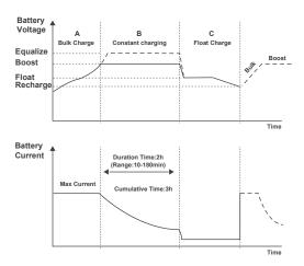
**Bulk Charge:** This algorithm is used for day to day charging. It uses 100% of available solar power to recharge the battery and is equivalent to constant current. In this stage the battery voltage has not yet reached constant voltage (Equalize or Boost), the controller operates in constant current mode, delivering its maximum current to the batteries (MPPT Charging).
